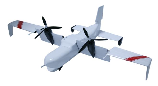
The AT-10 is a versatile small UAS designed for significant range and payload capacity with operation from shipboard and austere airfields. It is vertical takeoff and landing capable, and can also take off and land as a fixed-wing aircraft from short fields. It transitions to fixed-wing forward flight for climb and cruise, and can quickly transition from forward flight to hover to observe nimble ground targets.
